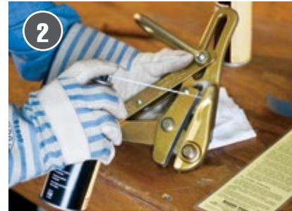
▲ **Step 2.** Spray degreaser on the grip jaws, all joints and moving parts
