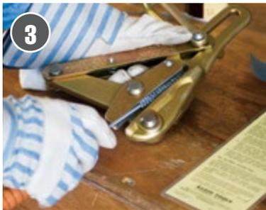
◀ **Step 3.** Use the Klein Grip Cleaning Wire Brush to remove dirt and debris from the grip jaws
