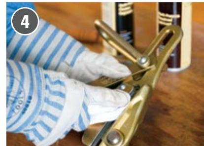
**Step 4.** Wipe grips dry with soft cloth. ▶ Repeat all cleaning steps as necessary until grip is completely clean
