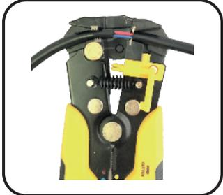
Strip the outside jacket of multi-strand irrigation cable without touching the inside cables
